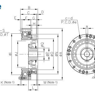
Note 1: The structure design of the section shall be left aside according to the suggestions on the diagram, so as to avoid the influence on the performance and service life of the gear reducer.
